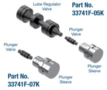
wear at the inside of the lockup control plunger valve sleeve allowing oil to escape, which affects the timing and quality of the lockup clutch apply and release action.
