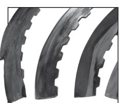
Figure 1 Broken OE Waved Plates
