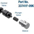
select switching valve and is also influenced via apply and release feedback balance passages. A worn bore, valve spool(s) or plunger valve assembly can cause loss of critical pressure to the sump, lube circuit or directly into apply or release passages, resulting in jerking on coastdown, harsh engagement and high engine RPM due to no lockup.
